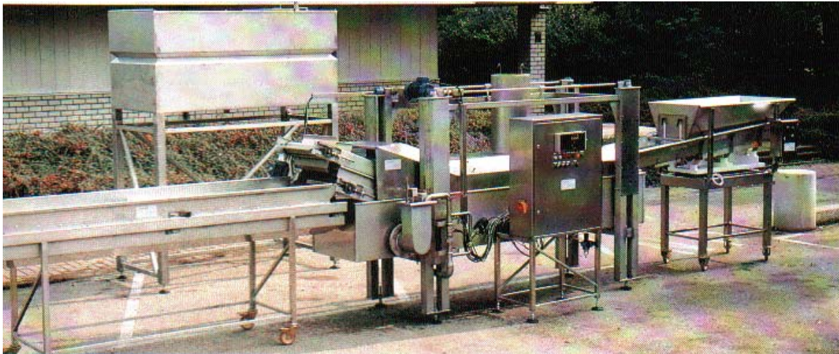
Pellet frying line 500 kg/hr
